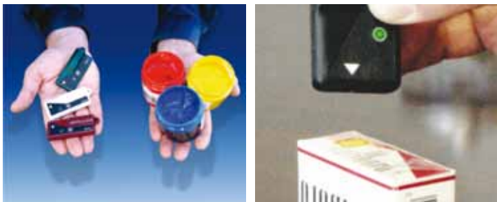
Using optical taggant inks and detectors (left) on packages (right).
