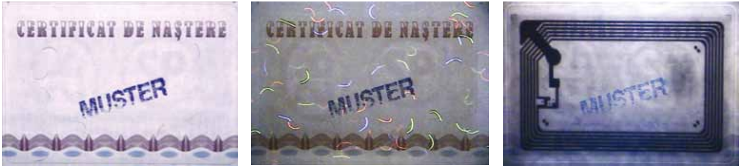
Figure 1: An image with covert security features viewed under (from left) visible, ultra violet (UV) and infra-red (IR) light. ]
